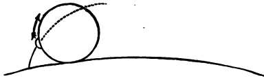
Fig. 2.—Generating Circle tracing Epicycloid for Wheel Tooth by rolling on the Pitch Circle.
